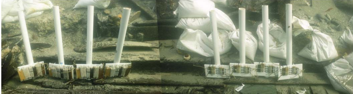
Fig. 6. The sacrificial wood and iron samples on the Clarence site prior to reburial. (J. Parkinson).
